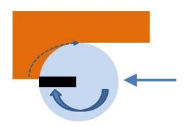
As for conventional milling but the chip will start out thicker and end up small.
