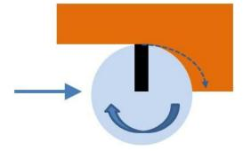
Each flute will carve out a chip from the stock as shown by the dotted line due to the movement and rotation of the flute as it turns and moves. The chip will start off small and get thicker as the bit moves and rotates.
