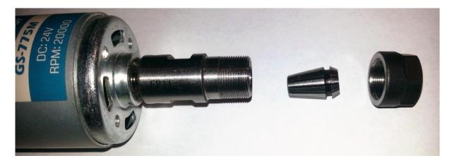
It has 3 parts, Holder, Collet and Clamping nut:
